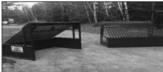
TR6 model , Our smallest model-designed for sub Compact tractors and other light duty Equipment. 2" minus fixed bar
